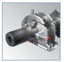
A cam-action spring tension holding device allows quick, easy and equal adjustment of the tension on all springs simultaneously from one end of the door. The cam tensioner bites into the axle helping to eliminate the unwanted spinning of the axle during the initial spring loading or adjustment process.
