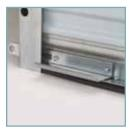
The slide bolt lock assembly affixed to the bottom bar at each end of the door curtain fastens through the guide to securely keep the door locked and in the down position. Padlocks can be attached to the slide to further secure the door.
