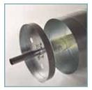
The 12" enclosed barrel houses the dead axle assembly and protects the factory lubricated springs from direct contact with environmental elements. The inherent strength provided by the spiral barrel minimizes axle deflection, providing smoother operation. Because the curtain is attached by screws and not seamed to the barrel, replacement of either independent assembly is cost-effective, guick and easy.
